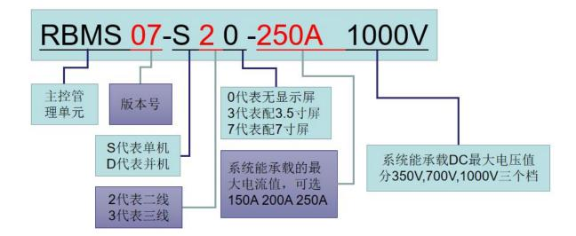
Example: RBMS07 D37-250A 700V represents that the GCE series BMS supports parallel, three-wire system, with a 7-inch display, and supports a maximum current of 250A and a voltage of 700V.
